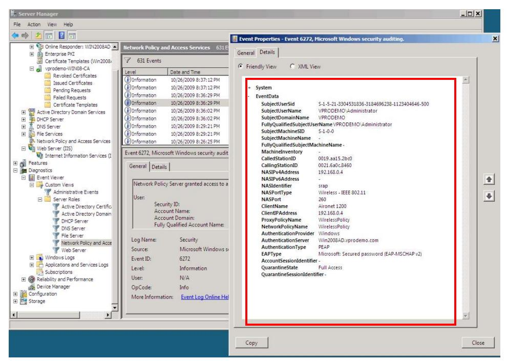
Notice the IP address of the wired and wireless configuration here.
